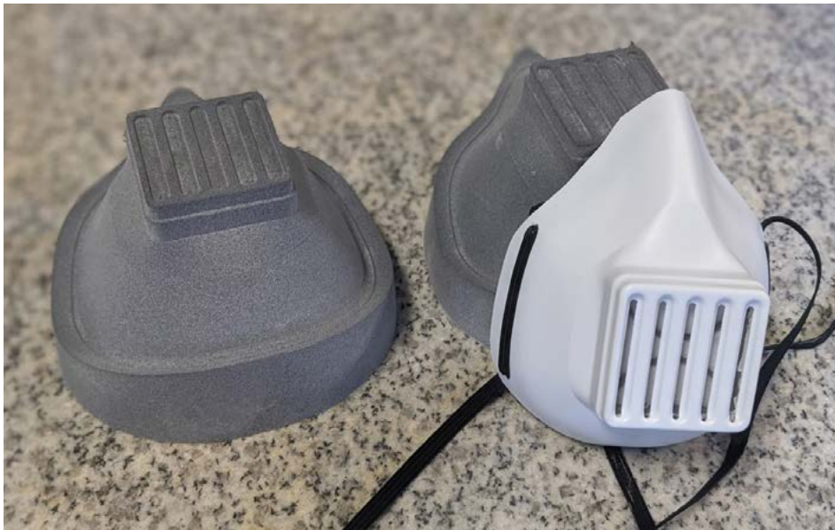
RapidMade began producing printed tooling for protective masks for the COVID-19 pandemic. As customers provided feedback, improvements were quickly made to the tooling. Courtesy of RapidMade
